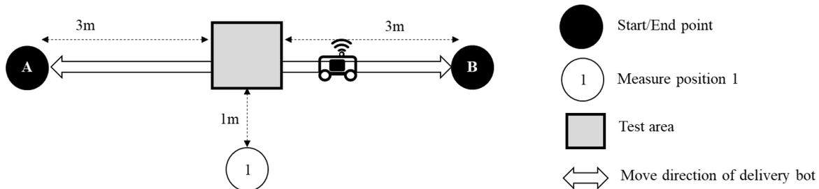
Figure 4 Experiment processes at position 1
